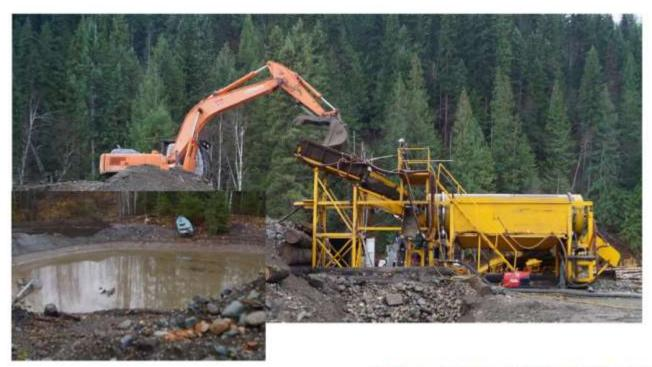
Settling pond, sluice box, and sluice machines
